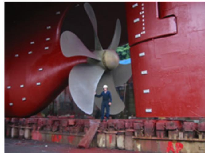
**Blades of propellers and turbines are chiral, therefore there is coupling between twist and bend deformations!**
