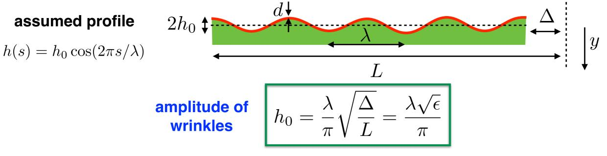
deformation of the soft substrate decays exponentially away from the surface
