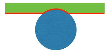
Wrinkling reduces adhesion (smaller contact area)
