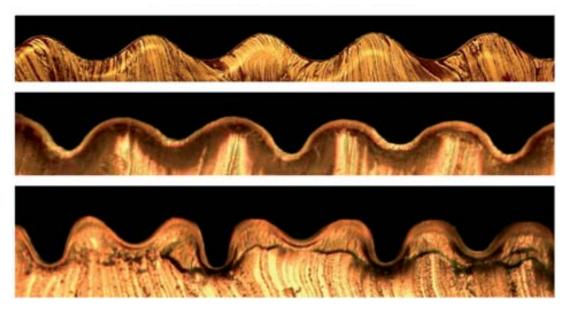
In order to explain period doubling (quadrupling, ...) one has to take into account the full nonlinear deformation of the soft substrate!
