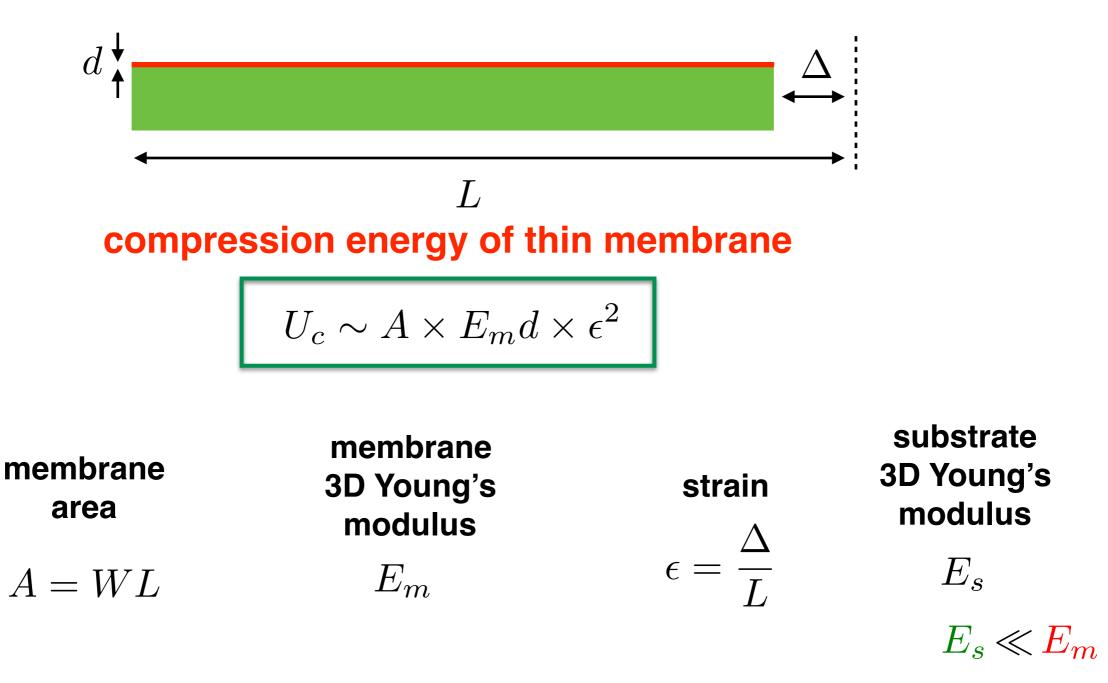
Note: soft elastic substrate is also compressed, but we will measure the substrate elastic energy relative to this base value!
