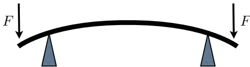
FIG. 3. (Color online) Edge torques acting on a membrane. The part of membrane that lies between the triangular supports, is influenced by external torques connected by a moment arm to the support. Torques are the consequence of external forces F acting on the sides of the membrane that lie outside the supports.
