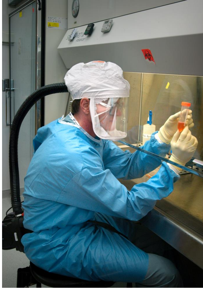
Figure A.1: Powered Air Purifying Respirator (PAPR) in use. A scientist handling reconstructed 1918 Pandemic Influenza virus in 2005 wears a PAPR. Fresh air in this PAPR is supplied to the head and face area via a tube connected to a fan and filter at the wearer's back. Photograph from Centers for Disease Control and Prevention's Public Health Image Library, public domain.
