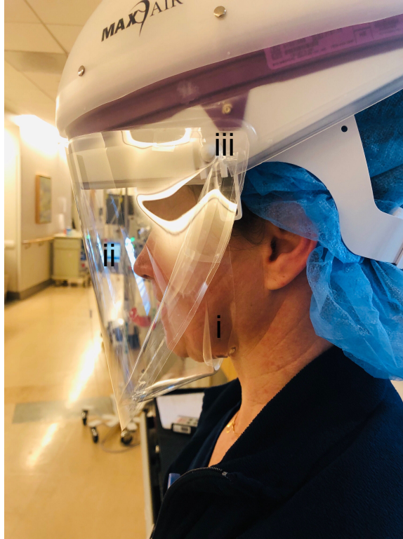
Figure A.2: MaxAir PAPR. Medical professional wearing the MaxAir PAPR with PAPR face shield made by Princeton volunteers. Face shield features a stretchable membrane (i) transparent face cover (ii) and attachment holes (iii).
