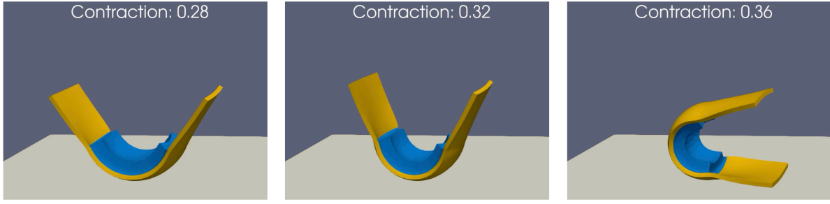
Figure 4.15: The self-folding unit deforming as contraction of the active layer (blue), g_i , increases in magnitude, left to right. The intermediate equilibrium state achieved at g_i = -0.32 maybe unstable and by adding perturbation in displacement before evolving the next steps we see that the structure topples and consequent equilibrium states are stable.
