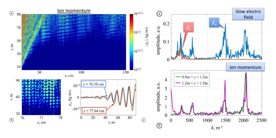
After the HF dynamics is filtered out, well-defined peaks in the spatial spectrum of the electric field and ion-momentum field are identified in the LH range.
