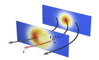
Narrow beam: one reference ray + diffraction. Having no crossing rays means having no caustic issues.
