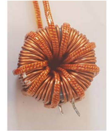
Rectifier-Coupled Boost Inductor N_A: 1.1\Phi, 72 \text{ turns} N_B: 0.05\Phi \times 320, 8 \text{ turns}
