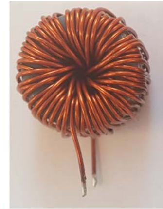
Conventional Inductor N_A: 1.2\Phi, 72 \text{ turns}
