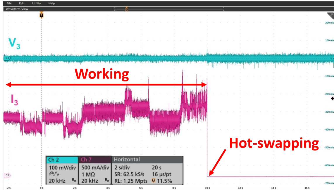
Fig. 25: Transient response when removing all 5 HDDs from one voltage domain (Port #3) at HDD server.
